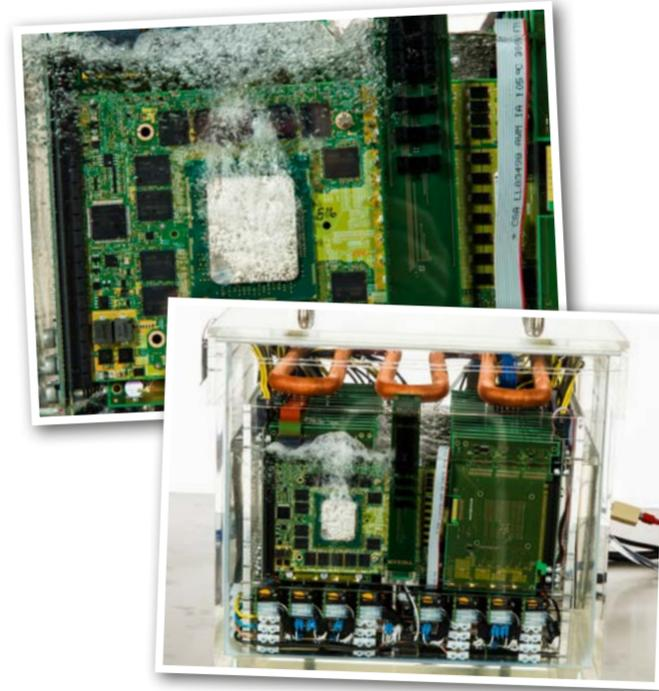
This concept prevents the components that are heating up from coming into contact with the ambient air. This results in an enormous energy saving potential for the air conditioning of computer rooms. No heat is emitted into the computer-center or work-area rooms. Blowers, air-conditioning and ventilation equipment can be almost entirely eliminated.
