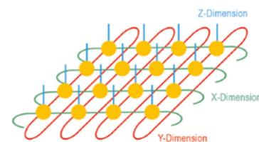
The entire Booster system thus encompasses a total of 32 nodes. The peak computing performance of the system is 38.4 Tflop/s. One layer (X-Y level) of the EXTOLL infrastructure is shown in the graphic.
